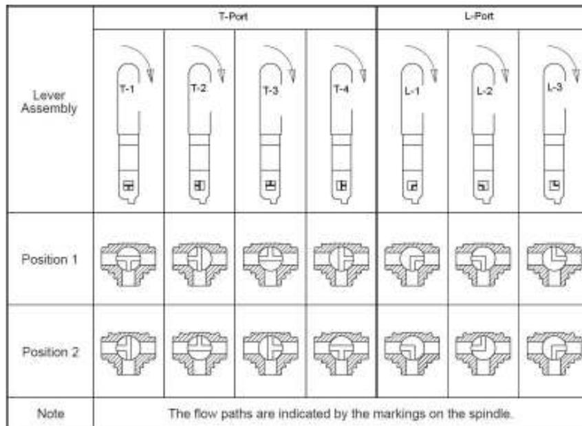
Chart Showing Flow Path of 3 Way T-Port and L-Port Ball Valves
